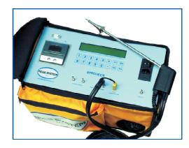
Polycarbonate keypad with large backlight LCD display
